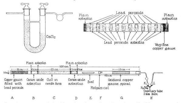
ing, is recommended. For the absorption of carbon dioxide two usual U-tubes filled with soda lime are employed.
